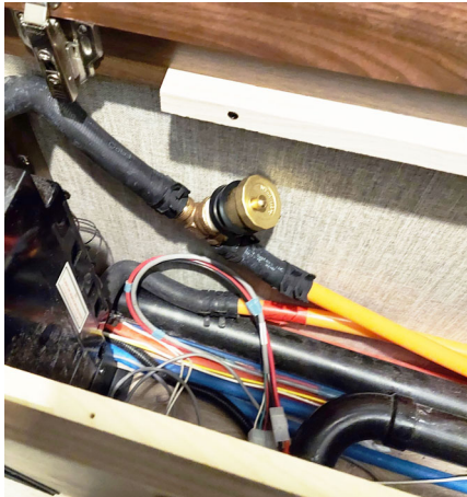
Example of second pressure relief valve in motorhome (N40P shown) -Typical View
