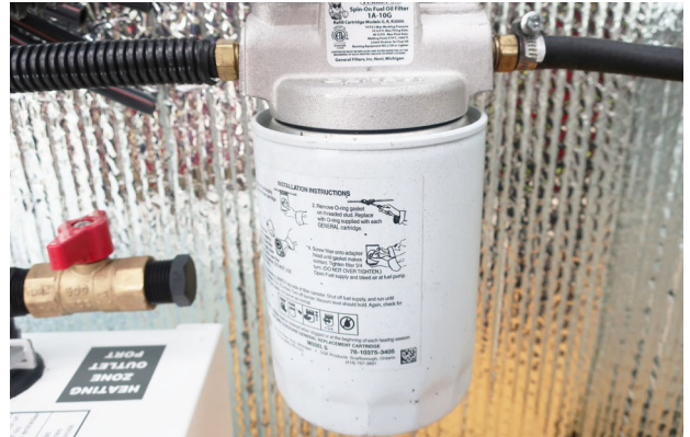
Aqua-Hot Fuel Filter (Located in center of motorhome behind front wheels) -Typical View
