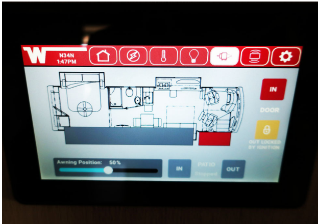
Awning Control Switches (Located in the slideout menu on the systems monitor panel) -Typical View
