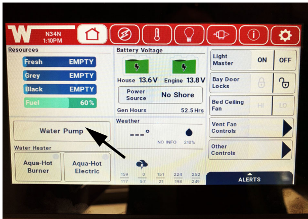
Water Pump Button Tap Water Pump to turn off/on -Typical View
