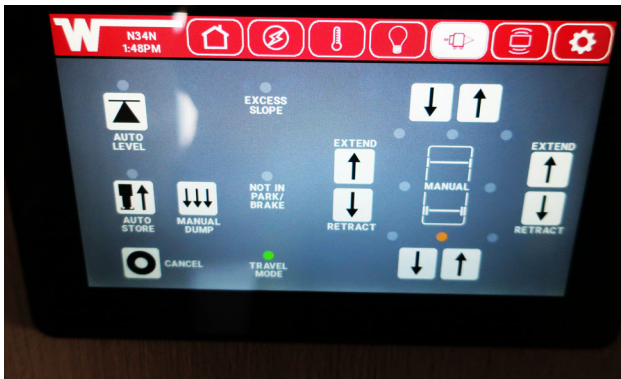
Leveling System (Can also be located in the monitor panel) -Typical View
