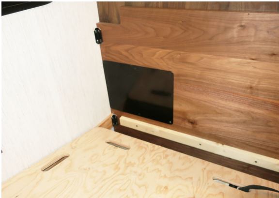
Locate and remove the access panel on the passenger side interior. -Typical View
