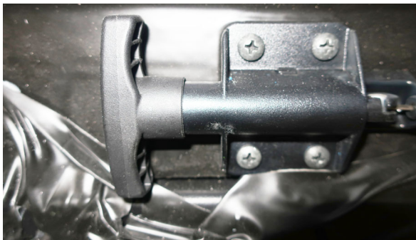
Power Compartment Door emergency release lever- pull to release corresponding door. -Typical View
