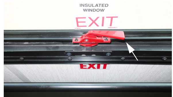
Escape Window (Lift red safety latch handle UP and push window OUT) -Typical View
