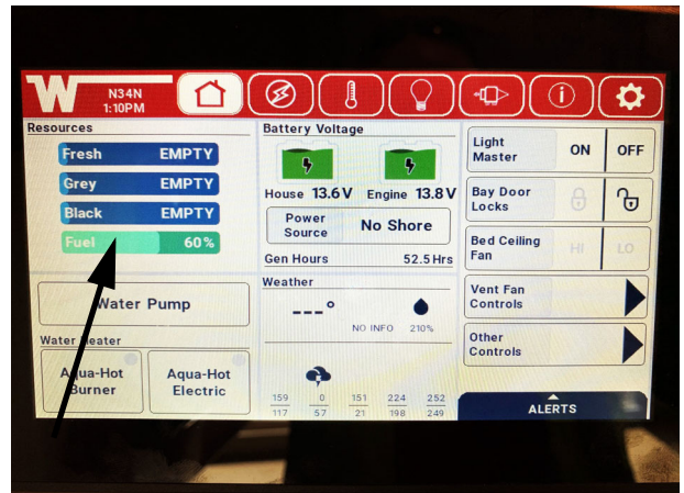
Holding tank levels on the Home Screen -Typical View
