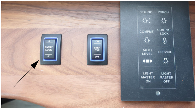
Power Door Locks - Entry Door (Located on the passenger side control panel)
