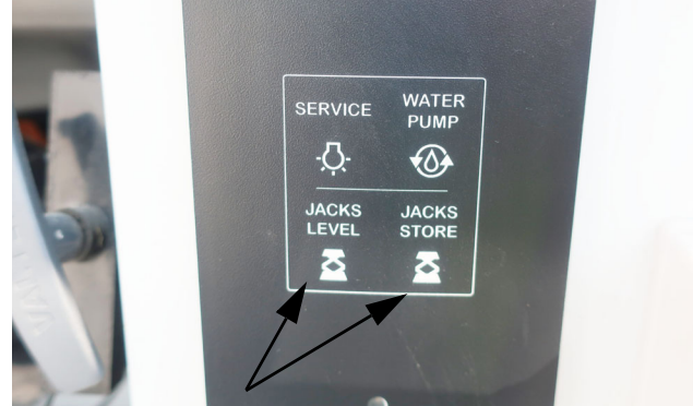
Auto Level Remote Switch (Located in the water center compartment) -Typical View
