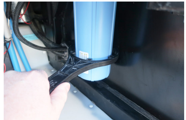
Use the Filter Wrench to loosen the filter, then unscrew it -Typical View
